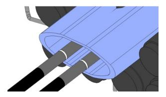
Push the seal upwards to the base and mark the cable flush with the seal. Make sure the seal touches the base.
