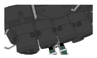
Adjust the orientation of the seal for better access to the two fixing points.
