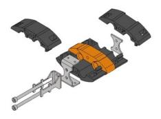
Open and remove the oval shells unscrewing the two screws of the oval port sealing device.
