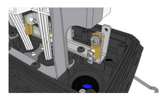
When drop cables have stength members, install the stength connectors to the frame in front of the chosen round port. Following the type of chosen seals, the corresponding connector is delivered within the bundle.
