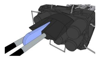
Push the seal against the base and set the melt welding clip. Start heating the seal on the base for one minute and shrink in spiral movements downwards around the seal.
