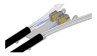
Insert the strength members of the cable into the connector on bracket such as all loose tubes can be routed without unnecessary crossings.
