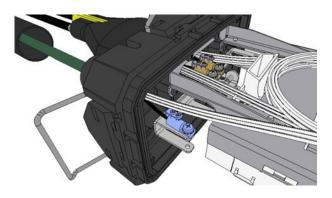
Push the cable into the opened round port and mount the connector onto the anchor support bar.
