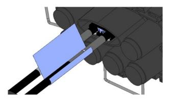
Place the edge of the aluminium protection foil 2 cm over the mark on the cable. Wrap it around the cable.
