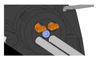
Seal the round port by tightening the screw with a minimum torque of 3.5 N.m.
