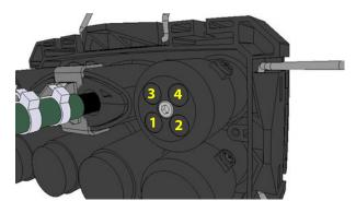
In case of multiple input seal, install the cables starting from the farest positions away from the edge of the closure.
