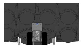
Push the device towards the base and fix it to the oval port, tightening the self-tapping screws.
