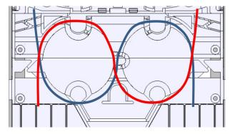
The block at the base of the frame routes the fibers from right to left and vice versa.
