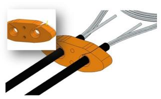
Install the looped cable into the grommet through the two cuts. The two cable jacket ends should protrude approximately 1 cm.
