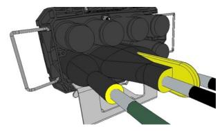
Push the seal against the base and start heating the seal on the base. Hold the cable in position. Shrink until the molten matter overflows from the extremity.
