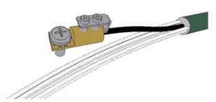
Insert the strength member of the drop cable into the connector and tight the screws.
