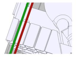
Match the loose tubes on the tube holders and mark at 1 cm over the edge.
