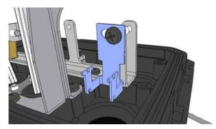
In case of a drop cable without strength member, install the bracket to the frame in front of the selected round port. Following the type of chosen seals, the corresponding bracket is delivered within the bundle.
