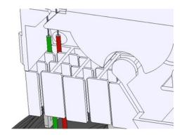
Remove the tube's sheath from the level of the mark and place them into the first available slot at the bottom of the device.
