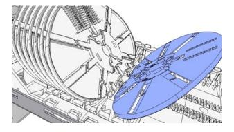
For trays of an height of 4 mm, install one tray on each hinge position of the base block.
