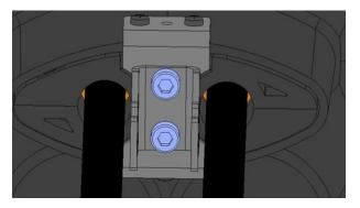
Seal the oval port by tightening the two screws of the device alternatively, respecting a minimum torque of 4.5 N.m.
