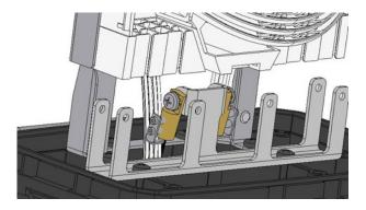
Fix the strength connectors to the frame avoiding unwanted twists with the tubes.
