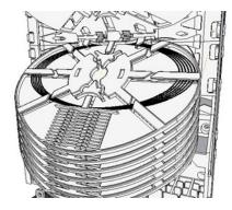
Gently guide the fibers up the respective splice tray and make sure that all the fibers are well positioned.
