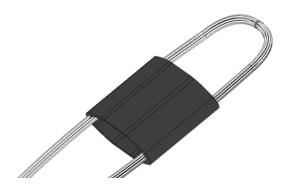
To prevent dirt and modules' grease to affect glue performances, put the packaging film of the sleeve into the latter. This will protect the internal lining. Bend the loose tubes gently and push them into the sleeve.
