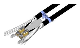
If the cable diameter is less than 10 mm, fix the cables with tie wraps. If the cable diameter is more than 10 mm, fix the cables with the hose clamp onto the bracket. Wrap few layers of tape around the hose clamp.
