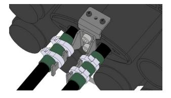
When the cable has a diameter under 10 mm, wrap velcro stripes on the cable and fix it with four tie wraps.
