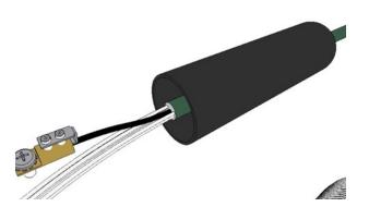
To prevent dirt and modules' grease to affect glue performances, put the packaging film of the sleeve into the latter. This will protect the internal lining. Push the cable gently into the sleeve.
