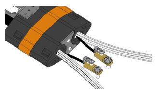
Insert the strength members of the cable into the connectors and tight the screws.
