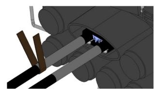
Abrade the jacket of the cable and the external surface of the port using a sand paper stripe.
