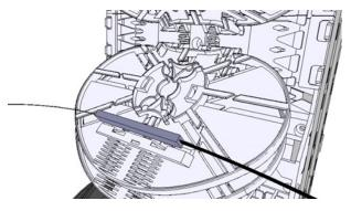
Splitters can be installed in a specific splice tray (part number CO522). Mount a PLC splitter (max 4x7x60mm) on the first side of the chosen tray.
