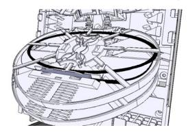
Dispose of the slack of the input and output fibers of the splitters within the tray. Identify the trays with a marker or a label.
