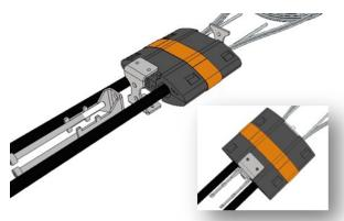
Finish the assembly of the device mounting back the plates and the screws. At this stage, avoid any compression of the grommet.
