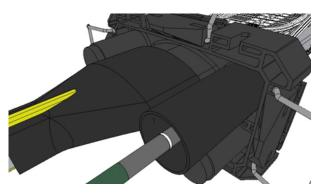
Push the seal upwards to the base and mark the cable flush with the seal. Make sure the seal touches the base.
