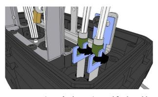
...or wrap a piece of velcro stripe and fix the cable to the bracket using tie wraps.
