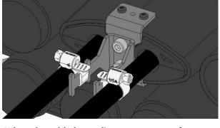
When the cable has a diameter over or of 10 mm, use two hose clamps to fix the cable to the bracket of the device.
