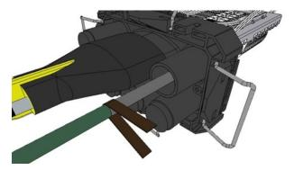
Abrade the jacket of the cable and the external surface of the port using the sand paper stripe.
