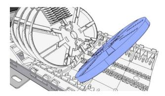
For trays of an height of 8 mm, leave one hinge position free between two consecutive trays.
