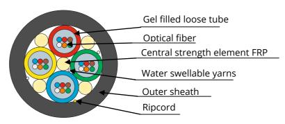
Cable consists of stranded core with central strength member (FRP), gel-filled loose tubes with optical fibers. Stranded core is fixed by water-swellable yarns. Outer jacket is made of polyamide PA12. Color of outer jacket is black. Ripcord is laid under the cable jacket.
